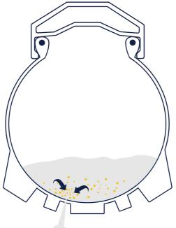
ALWAYS APPLY SEALANT WHEN THE VALVE IS AT 8 O'CLOCK POSITION.
